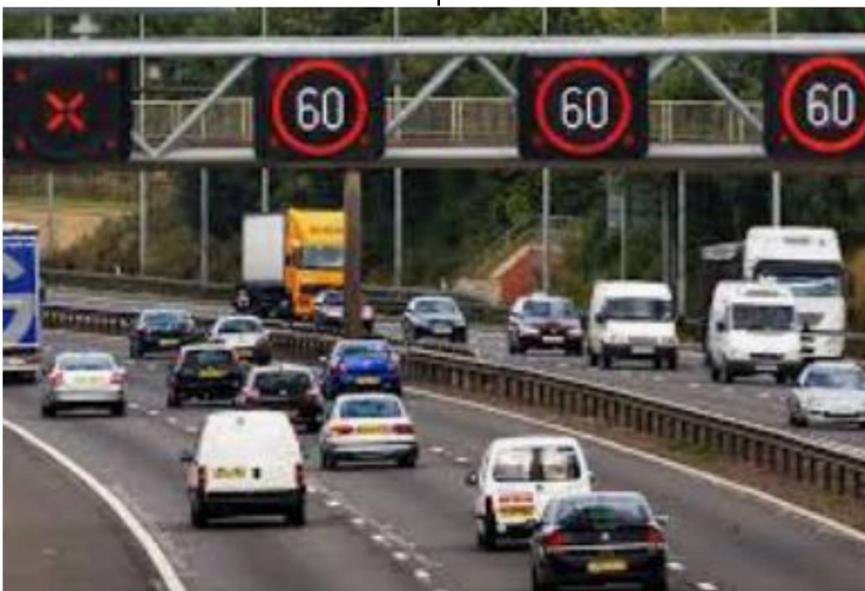
practice of drivers using lanes closed by a red X symbol on an overhead gantry. The signs are used when there is an obstruction such as a crash or
